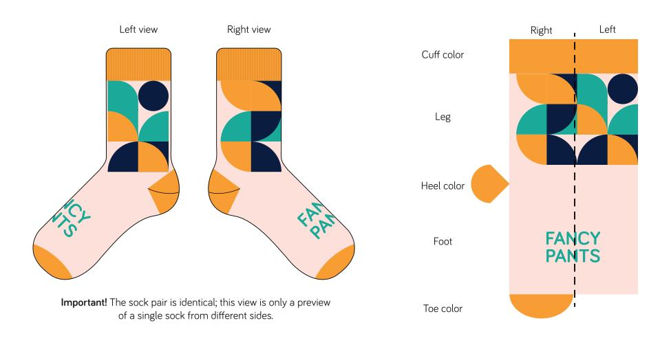
Parts that stretch the most are parts that you should avoid putting any graphics on instead of using a single color.
